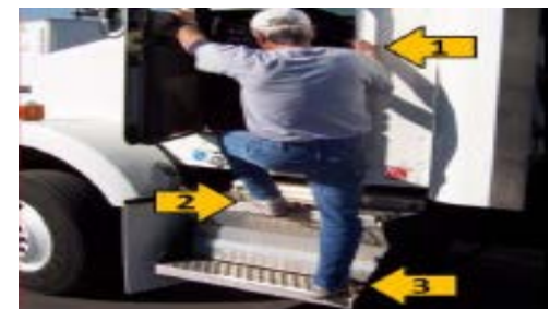
Always use three-point of contact when entering and exiting trucks.
